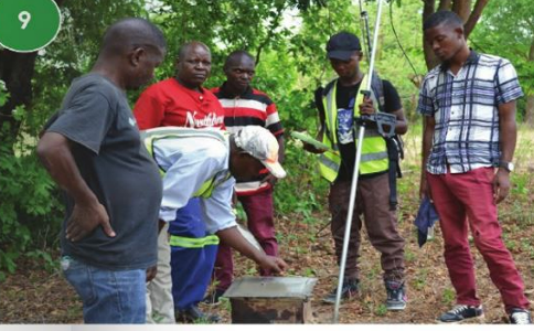
Picture 9: Physical planning officials erecting beacons during a boundary retracement process at Lengwe National Park
