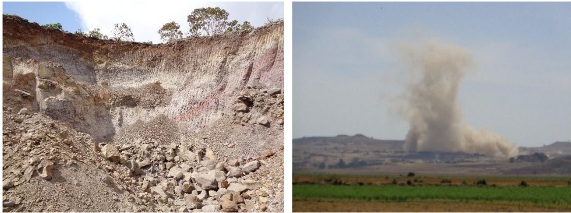
Figure 77" Borrow pit with dangerous steep slopes (left) and typical impact from blasting (right) (Source: BRLi, 2015)
