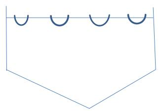
Two clarifiers have been provided in the design. Each of the clarifiers has a surface area of 6m x 4m and will be working together with the other one. During the cleaning of the clarifiers one clarifier shall remain on duty. The clarifiers shall be designed for a flow of 3,000 cubic metres per day. The design has provided for two clarifiers each with a surface area of 24 m2 and a depth of 6.5 metres. The clarifiers have been designed using the following formulae:
