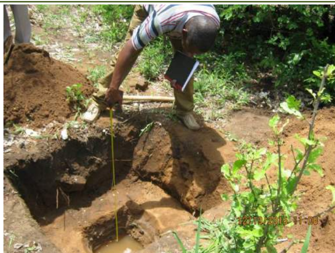
[Figure 2.3-7] Recording Time Taken for the Water Level to Drop to 225 mm
