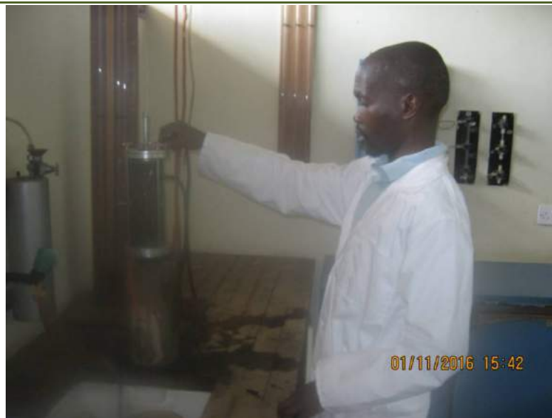
[Figure 2.3-9] Permeability Test
