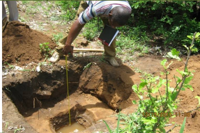
[Figure 2.5] Recording Time Taken for the Water Level to Drop to 225 mm
