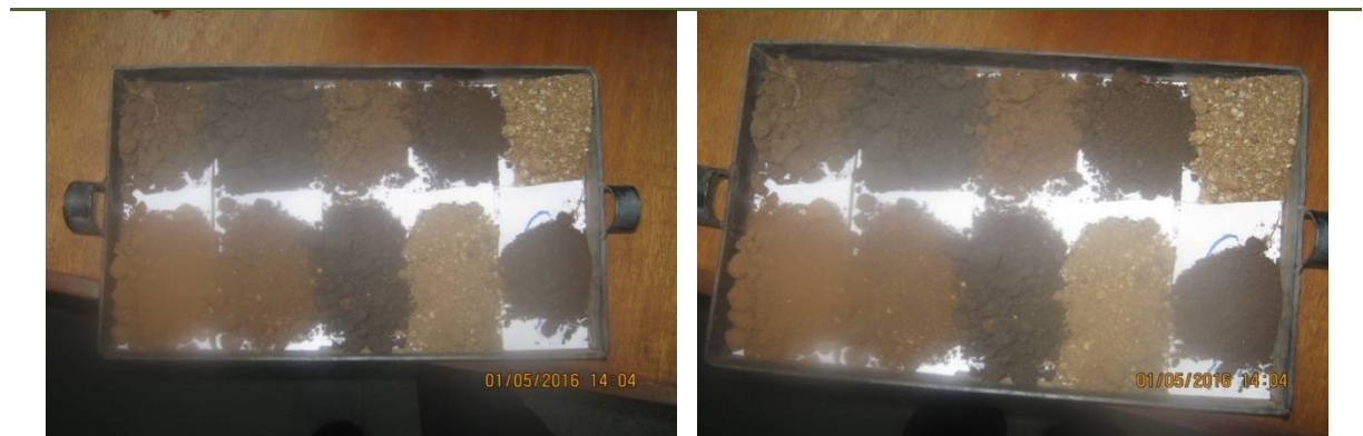
[Figure 2.8] Soil Samples Collected from the 10 Points on the Feeder Canal
