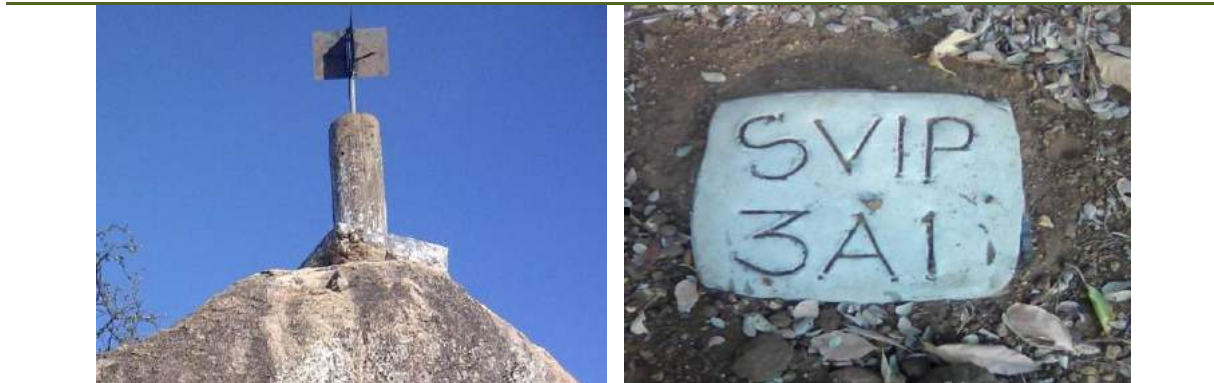
[Figure 8.1-2] Trig Pillar 318 NYS (Left) and Control Point Example (Right)
