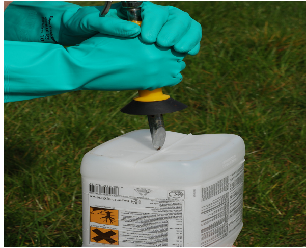
Figure 5: Pressure rinsing in action
