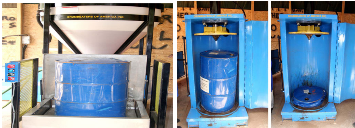
Figure 8: Automated solvent washing and crushing equipment
