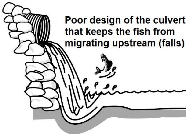
Figure 34 Poor design of a culvert
