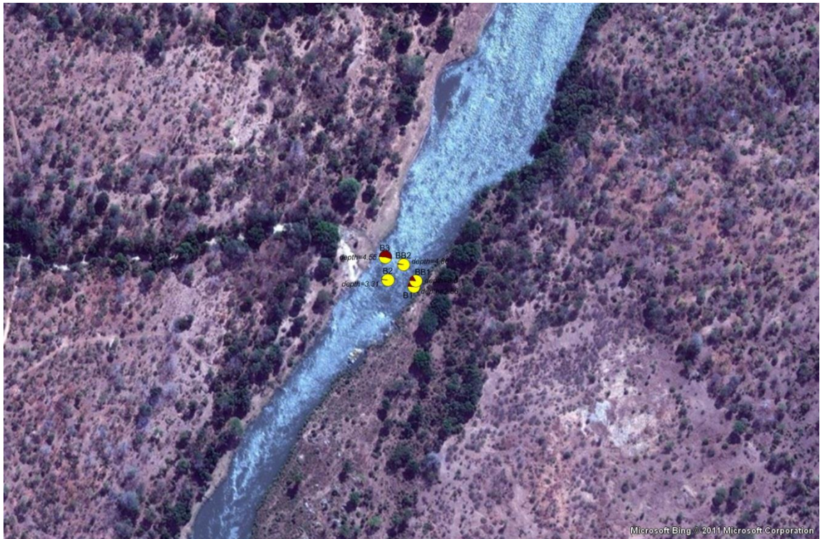
Fig. 14. Location and size-classes distribution of bedload samples – second survey – upstream of the reservoir
